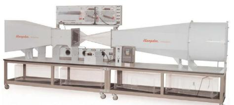
Model H-6910-12 Wind Tunnel shown with optional Experimental Packages Dimensions: 73"H x 180"W x 30"D, Weight: 2,000 lbs.
