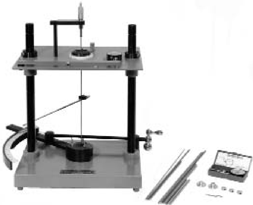
Model H-6311 Torsion Test Demonstrator Dimensions: 21"H x 19"W x 14"D
