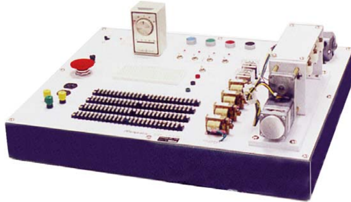
MODEL H-PLC-PP Peripheral Panel Dimensions: 9½" H x 26½" W x 22½" D Shipping Weight: 60 lbs.
