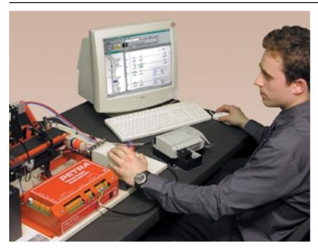
The PC55/ML teaching set introduces students to programmable controllers through a range of practical activities that are based on an advanced pneumatic/electronic applications trainer.
