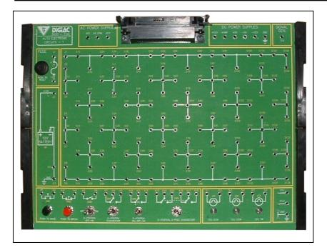
The D3000 7.00 Auto Electronic Circuits module allows students to build a variety of introductory automotive electronic circuits using a range of on-board and carrier-mounted components.
