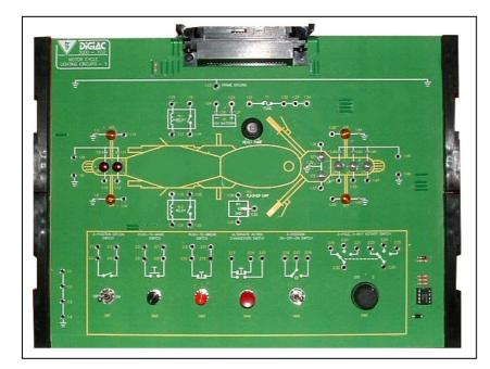
The D3000 7.02 Motorcycle Lighting Circuits module introduces students to the lighting circuits that are used on motorcycles.
